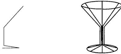
Fig.8.7: A model built by revolving a master contour about an axis.
